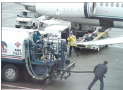
Nozzle screens should be checked for rubber particles that might indicate there is potential deterioration inside the hose.
