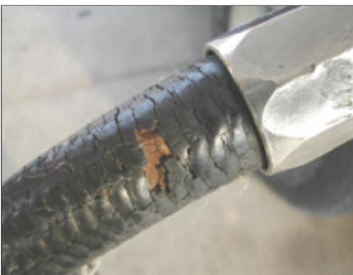
These requirements cover hose and hose assemblies (hose with couplings attached) in sizes up to and including 1-1/2 inches (38.1 mm). Dispensing hose is not permitted to be longer than 18 feet (5.48 m).
