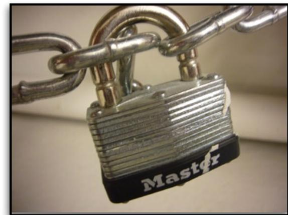
The shackle of this breakaway padlock is an example of a *frangible* element.
