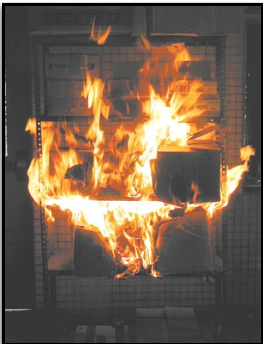
This shelf fire is an example of turbulent flame.
