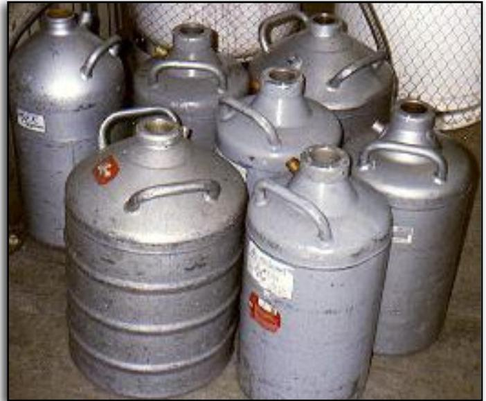
These metal carboys were used to transport cryogenic fluids.
