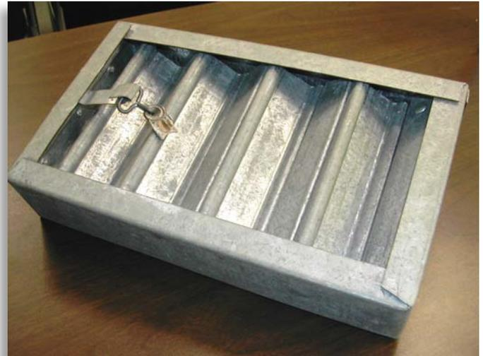
This fire damper has been released to illustrate its closed condition. One-half of the fusible link remains.
