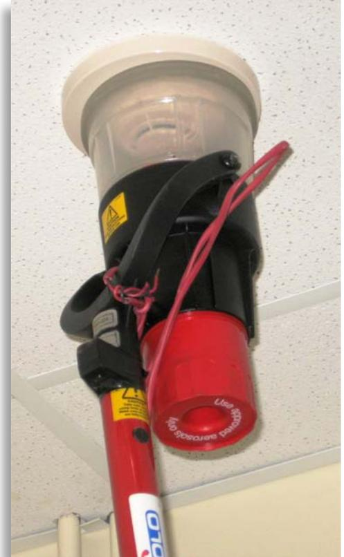
This testing device provides a calibrated release of artificial smoke. It tests detector performance and can be used to evaluate the sensitivity.
