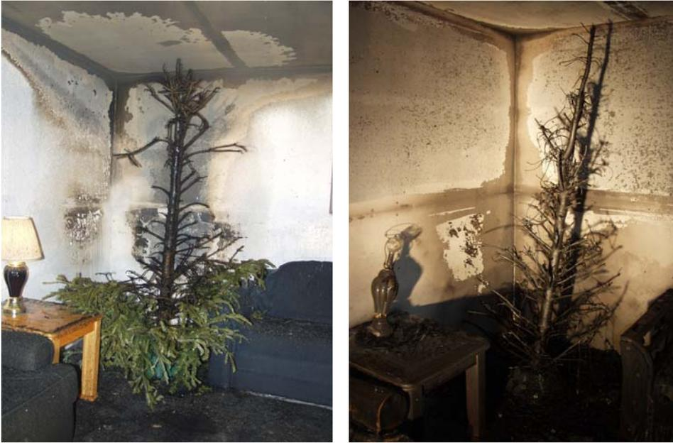
Figure 18. Post fire photographs (Sprinklered room on the left and non-sprinklered room on the right.)
