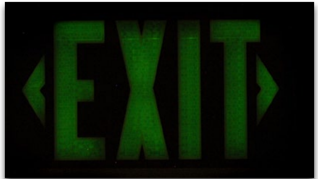
Figure 12. This photo shows the sign in the dark, with the glow visible. The Exit template and the prismatic lens are in place.
