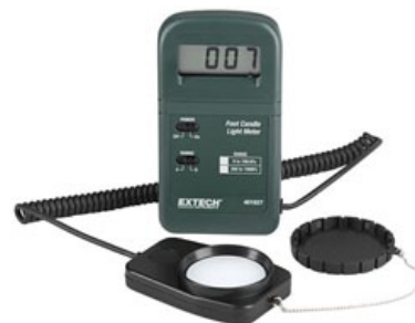
Figure 15. Digital Light Meter used to measure light level
