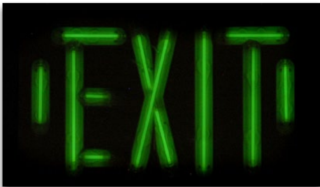
Figure 13. In this photo, the Exit template and the prismatic lens have been removed so that the tritium filled tubes are clearly visible.
